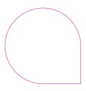
1: The contourline should have a line weight of 0.5 pt, the colour of this line must be a spotcolour called "cutcontour".
