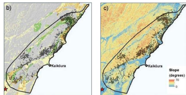
**Fig 1: Mapped landslides as of August 2017.** Inset map shows the area of New Zealand affected by coseismic landslides triggered by the M7.8 2016 Kaikōura earthquake. The main map shows the mapped (more than 11,000 landslides) coseismic landslide source areas and their size (area) triggered by the earthquake, superimposed on the 8m by 8m digital elevation model for New Zealand, classified by elevation in metres above sea level.
