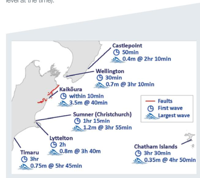
Kaikōura tsunami travel time map. From GeoNet tsunami gauges and Lyttelton Port Company and PrimePort Timaru tide gauges.
