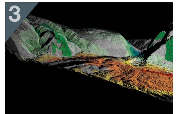
**Figs 2 & 3:** The images show the coloured point clouds from ground-based LiDAR surveys carried out of the Hapuku landslide dam by GNS Science. The left-hand image shows a model of the dam as it was in December 2016. The right-hand image shows a model of the dam in October 2017, after it had overtopped and breached. Note the breach geometry on the right of the right-hand image.
