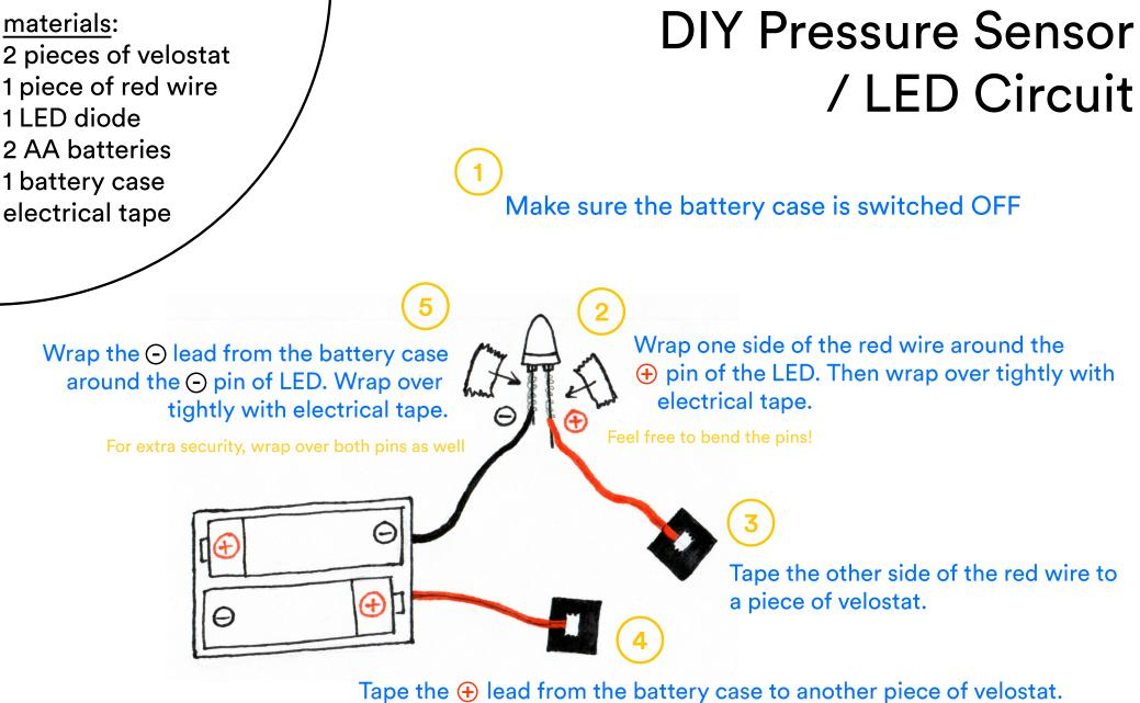
What happens when you squeeze the velostat pieces together? Velostat acts as a *resistor*, controlling the flow of electric current through the circuit. The more pressure is applied, the less resistance there is, resulting in a brighter LED.
